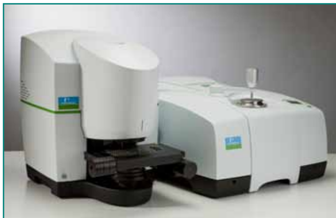
Figure 3: Frontier MIR/NIR with a Spotlight 400 mid-IR/near-IR imaging system.
