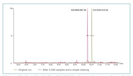
With its world-leading stability, the Clarus SQ  $8\,GC/MS$  can be returned to as-new performance levels with a simple, user-executable cleaning. In this example, note the chromatographic consistency for 1 picogram of OFN before and after the running of 2,500 high matrix environmental samples.
